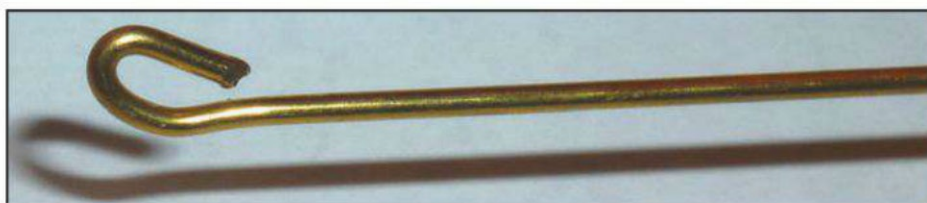
Photo F– Element tips should be rounded for safety's sake.
